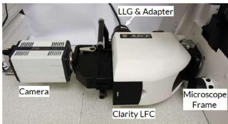
**Figure 5.1** Fully assembled Clarity system with Liquid Light Guide and collimating adapter, scientific camera and microscope frame.
