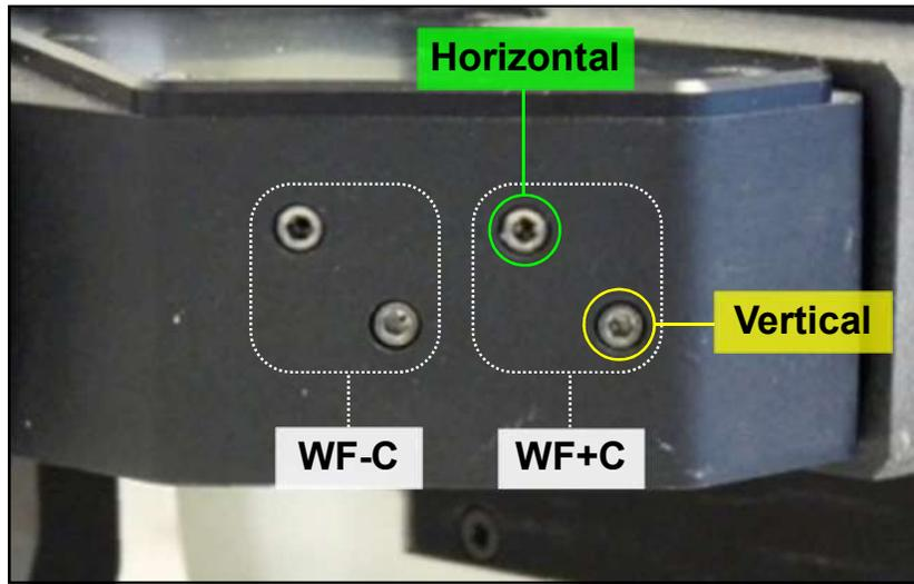
Figure 5.4.9(b) Camera alignment control screws
