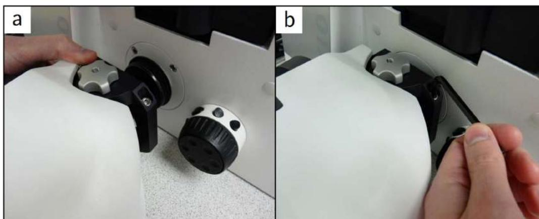
*Figure 5.4.2(a) Engaging Clarity onto the microscope adapter, (b) locking the microscope clamp.*
