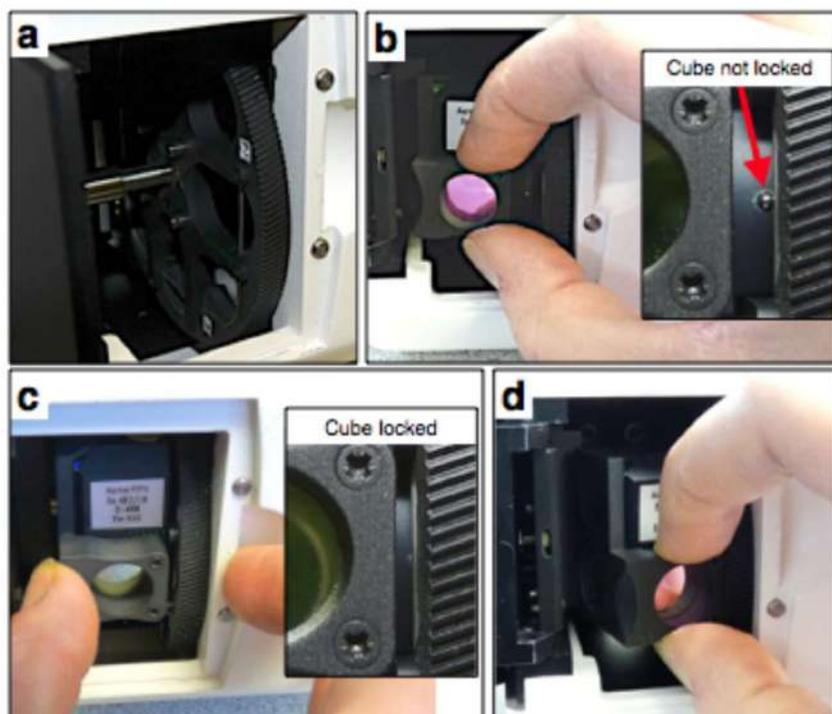
**Figure 5.4.4** Inserting and removing filter cubes: (a) filter turret, (b) filter cube insertion, (c) filter cube locking, (d) removing a filter cube
