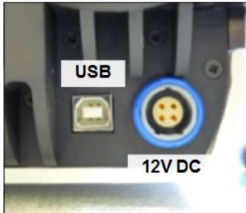
Figure 5.4.3 Clarity power and USB connections.
