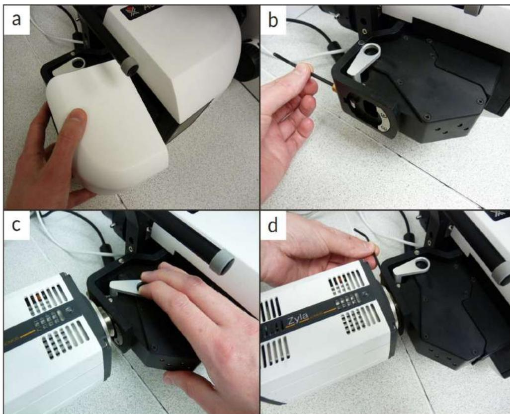
Figure 5.4.7 Attaching camera: (a) slide cover off, (b) unlock adapter, (c) attach camera, (d) camera adapter locking screw.
