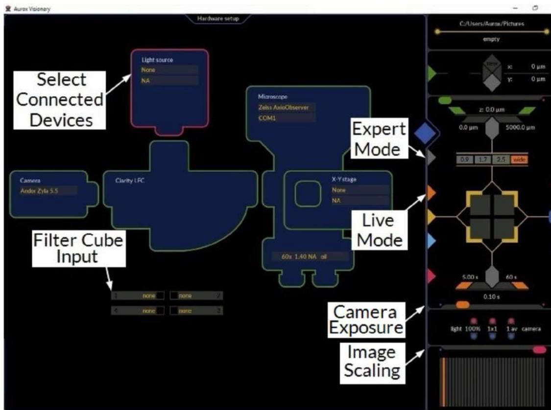
Figure 5.4.8 Visionary Hardware Set up Screen
