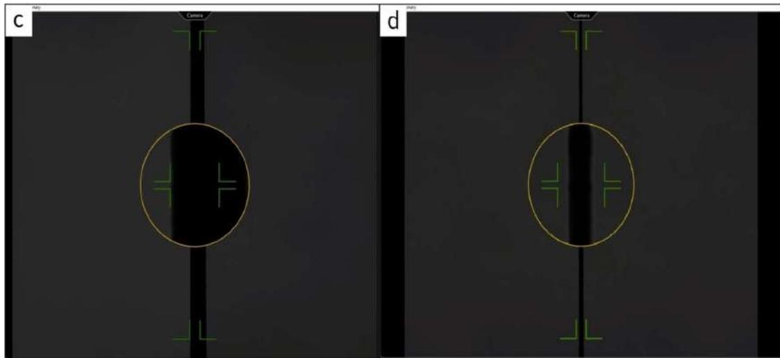
Figure 5.4.9 Alignment: (c) Camera aligned rotationally, (d) Images positioned
