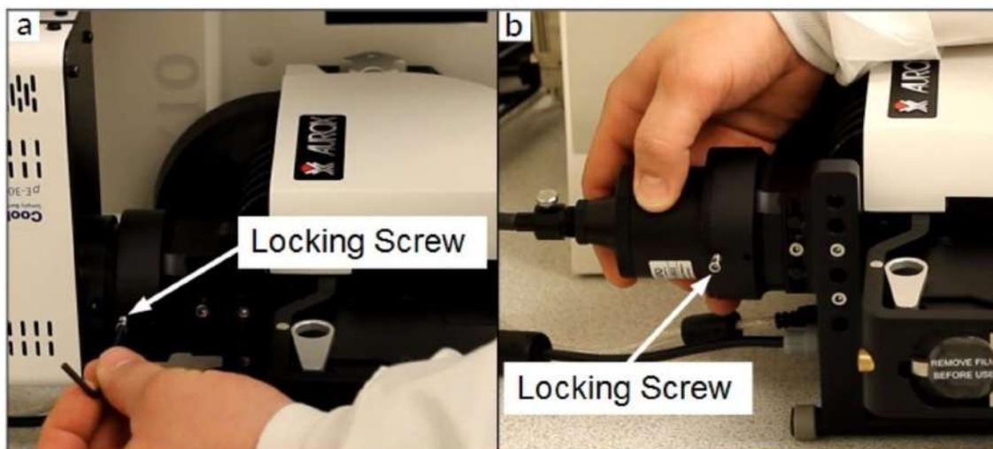
Figure 5.4.5 (a) Attaching a Light Source, (b) Direct coupling, Liquid light guide.
