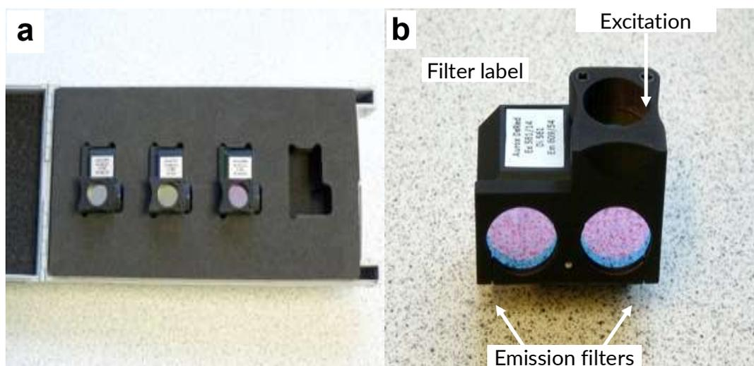
*Figure 5.2.1 (a) Filter cube case with three filter cubes, (b) Close-up photograph of a filter cube showing their positions and labelling.*
