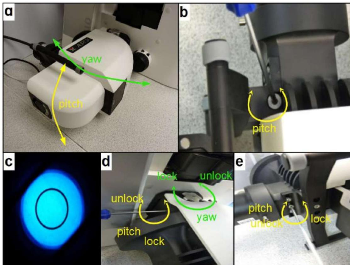
**Figure 5.4.6** Pupil alignment: (a) Yaw and pitch definitions, (b) pitch support leg adjustment, (c) correctly aligned pupil on ground-glass alignment tool, (d) microscope clamp pitch and yaw lock, (e) leg support pitch lock
