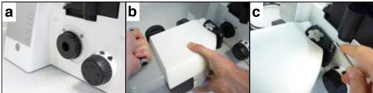
*Fig 3.3: a) microscope adapter fitted to the side port of an inverted microscope, b) Clarity LFC engaged onto the microscope adapter, c) locking the microscope clamp.*
